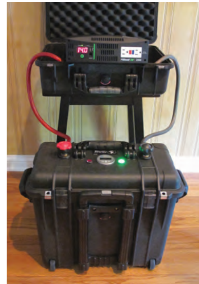
Powerenz. Custom solar-powered generators are built depending on how much power a user needs and how long a crew works. The units use LFP batteries, instead of the older lead acid technology, which makes them lighter in weight and 10 times longer lasting than other products, the maker states. Shown here is the LFP 200 Battery Module that has a monitor to display battery data and how many hours and minutes until the battery needs to be recharged. The time is based on a user's average power consumption over a three-minute time frame. 770.639.2244. www.powerenz.com . Circle 285.
